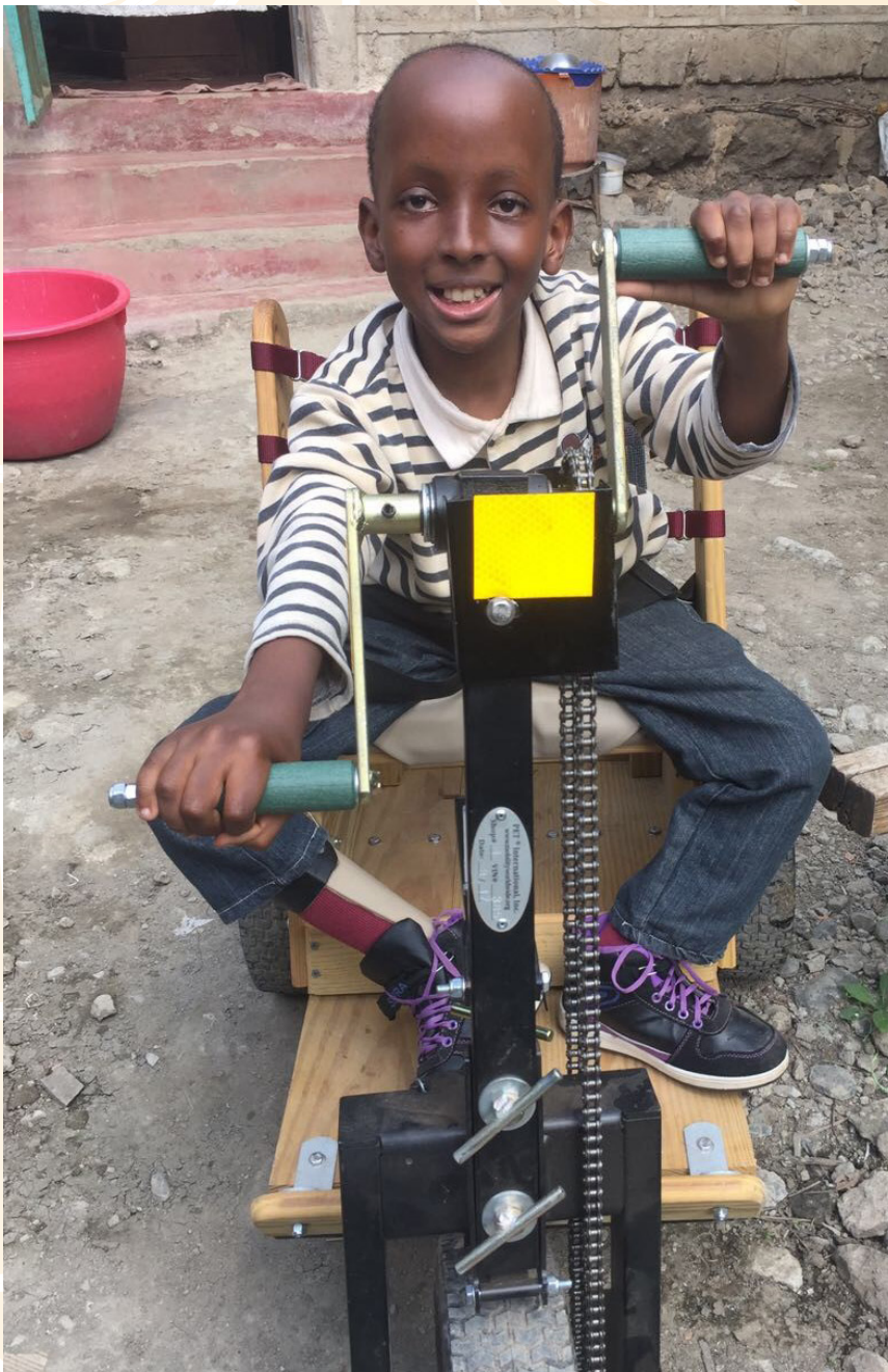
Small carts get overhaul in 2017. The seat was widened and the toe board was redesigned
